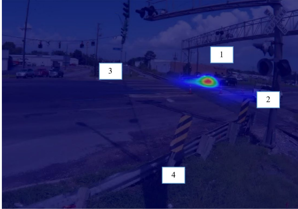
Figure 53. Louisiana Multi-lane Highway Grade Crossing Violator Spatial Heatmap for All Classes with Origin and Destination Zones (June 9, 2021, to June 26, 2021)
