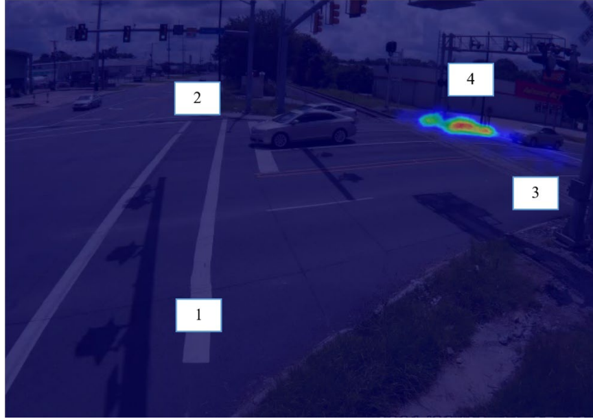
Figure 58. Louisiana Local Road Grade Crossing Violator Spatial Heatmap for All Classes with Origin and Destination Zones (June 9, 2021, to June 28, 2021)
