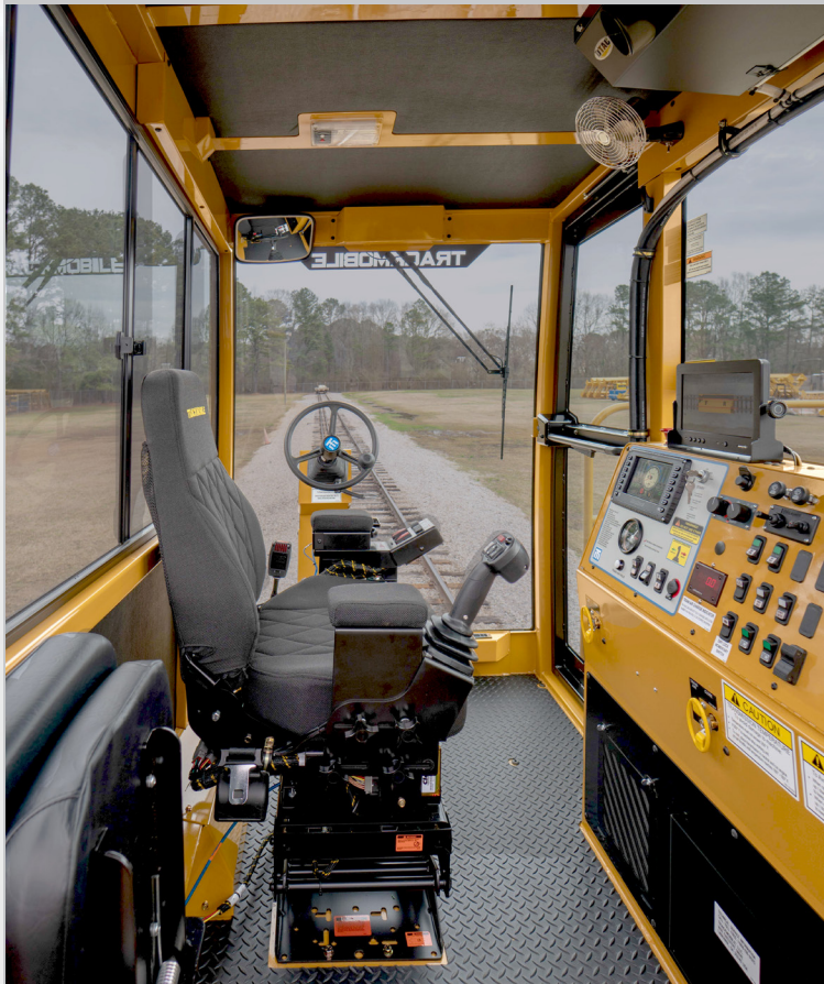
Atlas control panel and operational controls.
