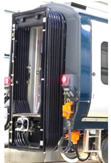
Image of Sealed Separable Passageways – Courtesy of CAF
