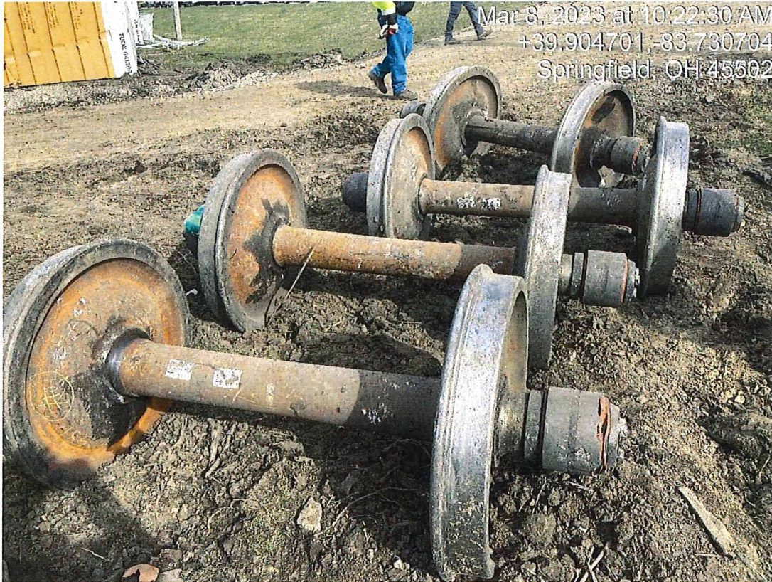
Figure 1. Wheelsets from car NS 162581 held by NTSB for investigation at the derailment scene.
