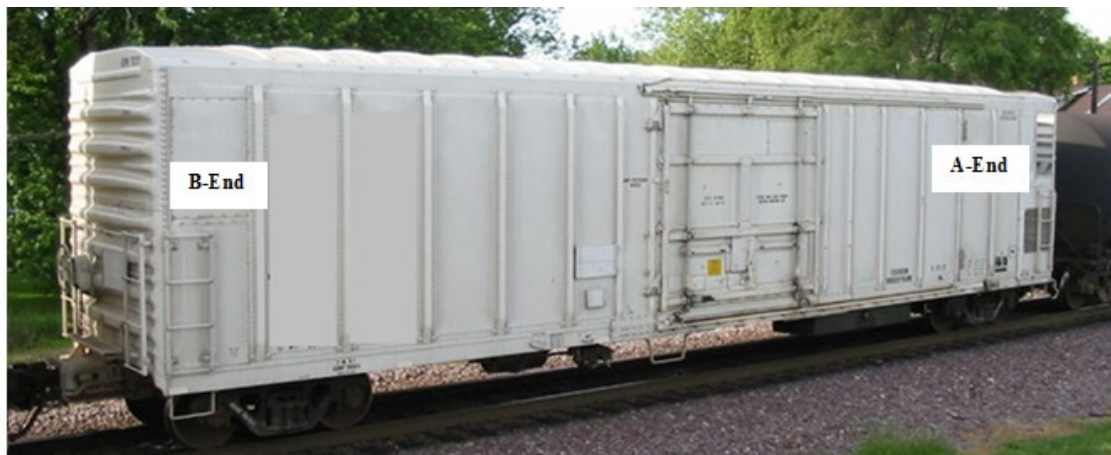
Figure 3. Typical Refrigerator Car
