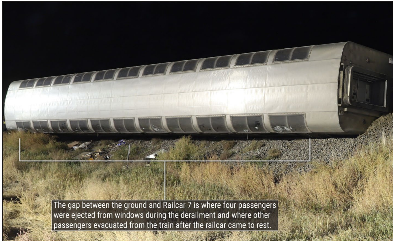
Figure 8. Photograph of overturned Railcar 7 in its position after the derailment.
