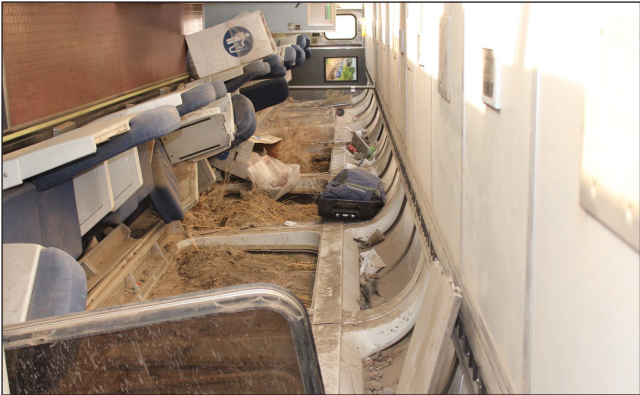
Figure 12. Interior of Railcar 7 after the derailment.
