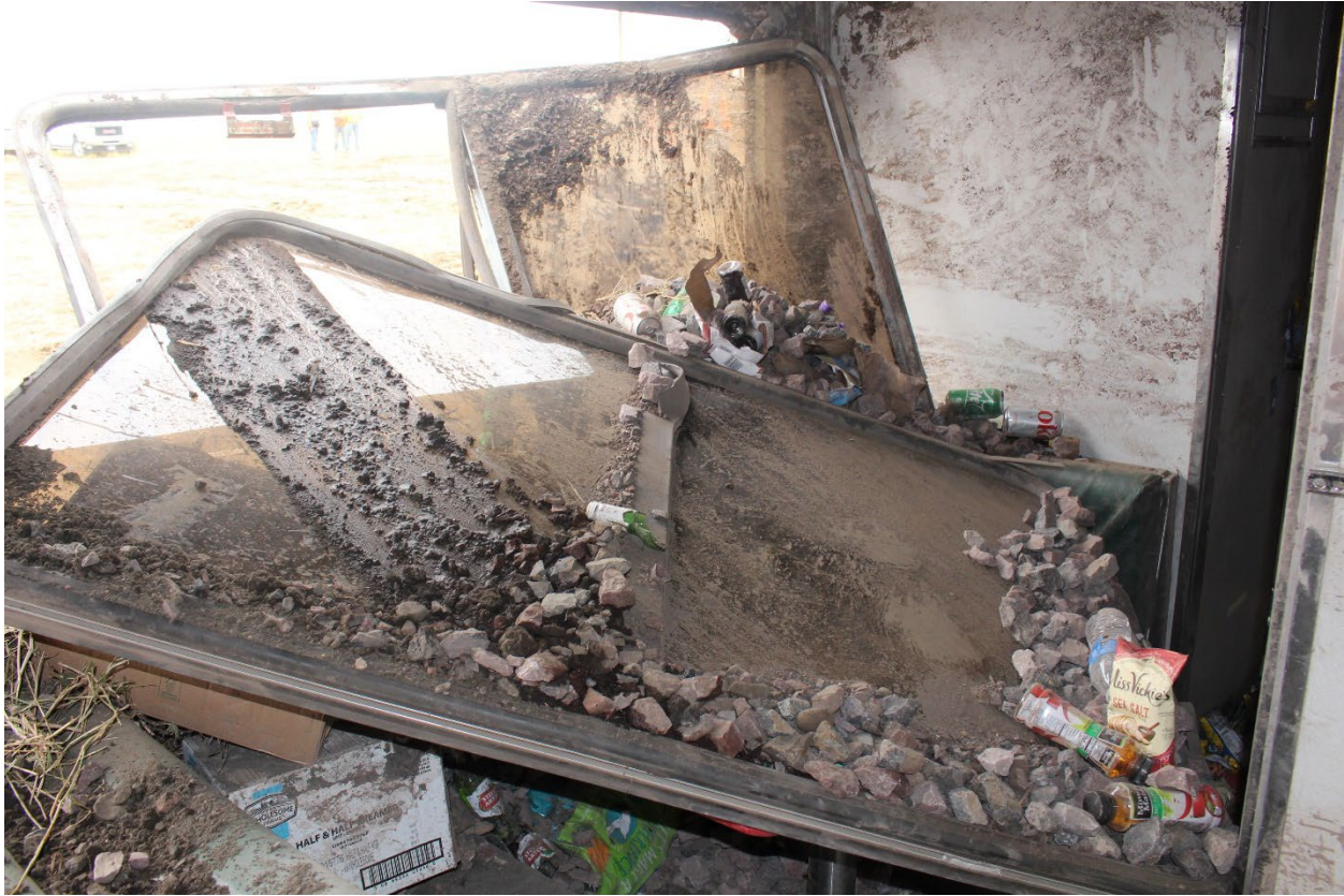
Figure 9. Postderailment photograph of a damaged window from Railcar 7.
