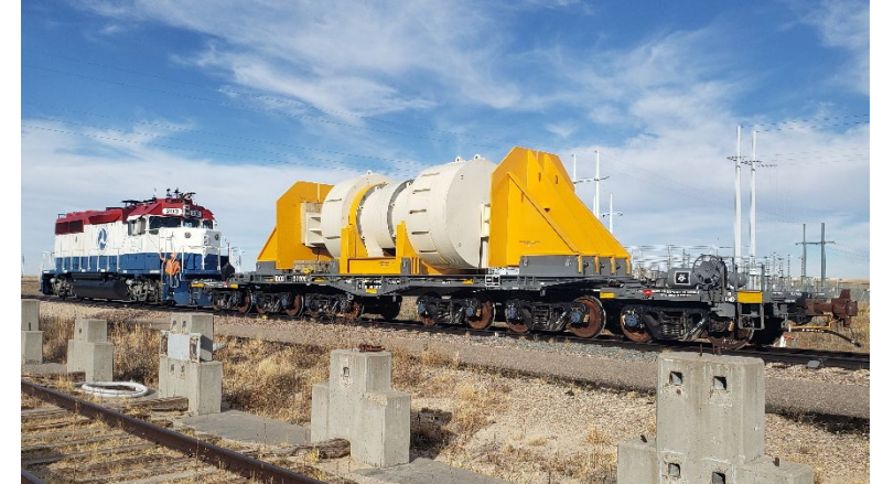
Photo: Atlas railcar with test weight
