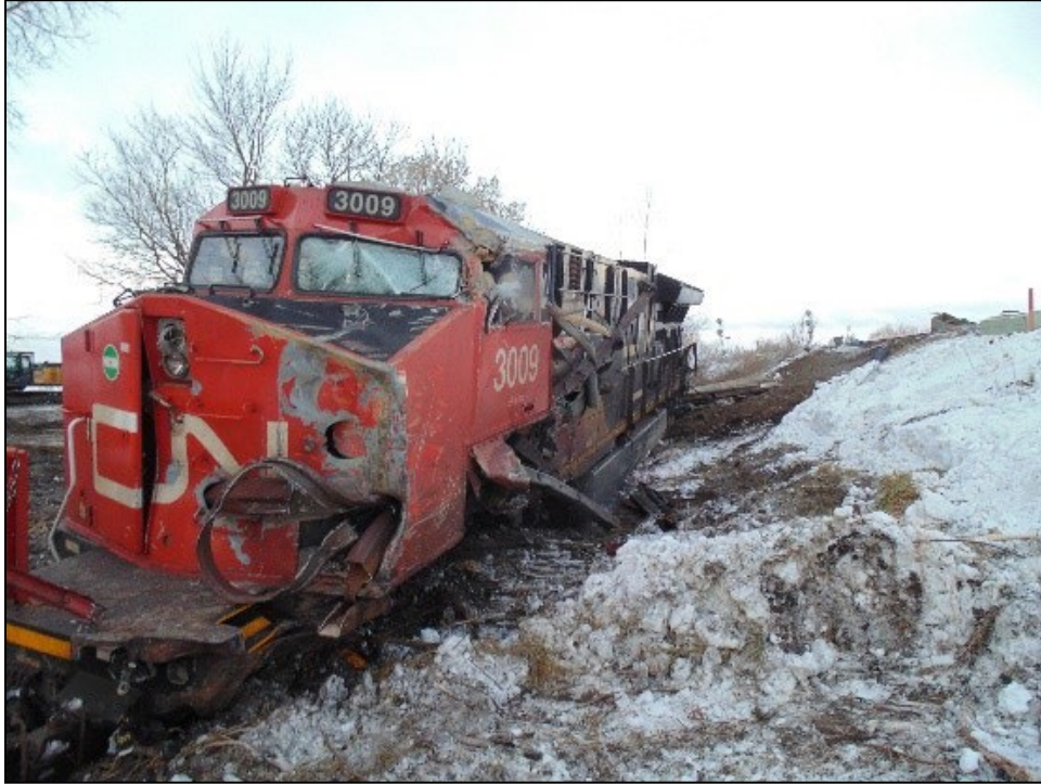
Figure 3. Damage to the north side of lead locomotive CN 3009 on train 318 (Source: TSB)
