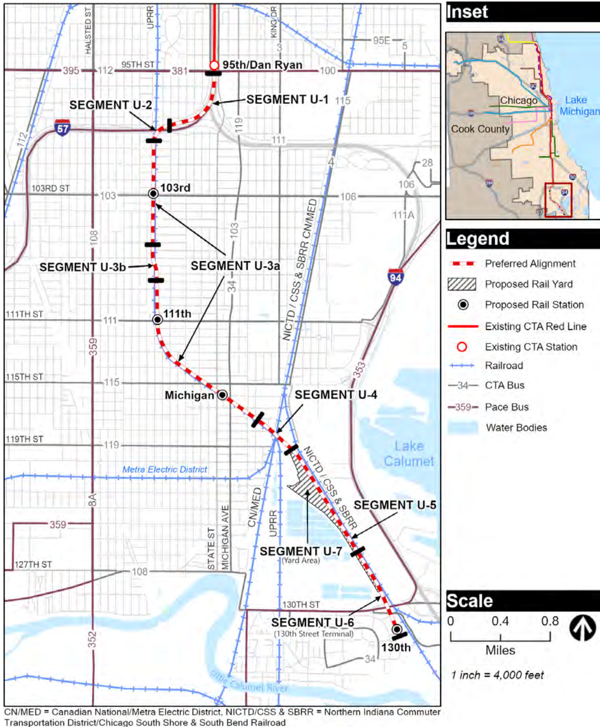
Figure 2-6: Construction Segments of the Preferred Alignment
