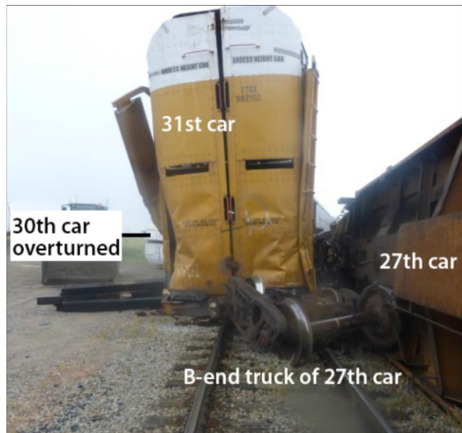
Figure 9. Leading end of 31st car TTXG 982102 and the trailing truck of 27th car (Source: TSB)
