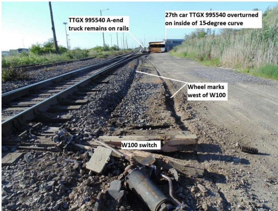
Figure 6. View southward from the W100 switch (Source: TSB)
