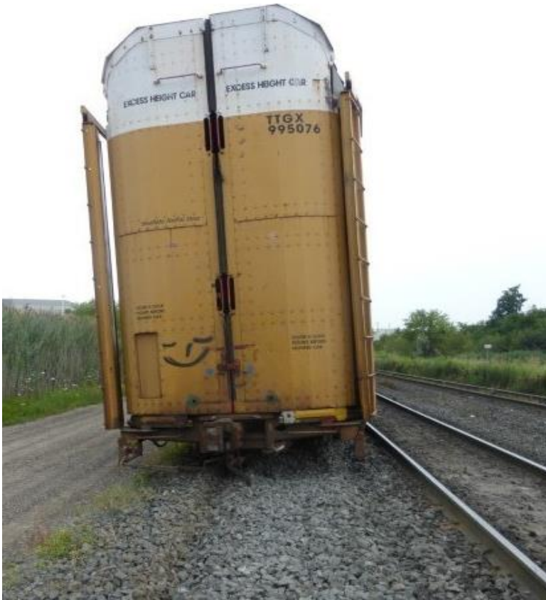
Figure 5. Trailing B-end truck of 26th car TTGX 995076 derailed; -end truck remained on the rails (Source: TSB)
