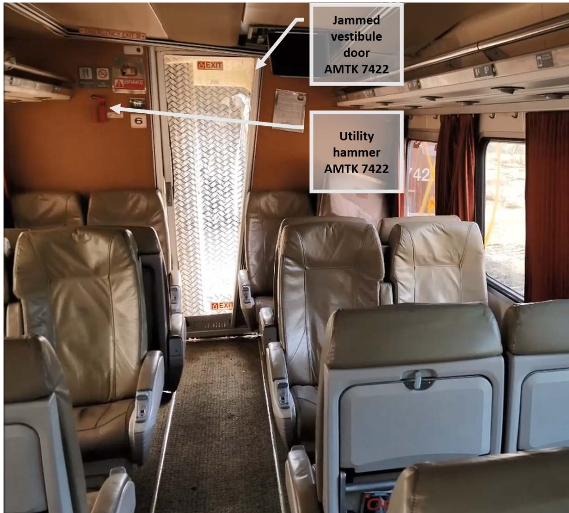
Figure 36. Jammed vestibule door, AMTK 7422 (10).
