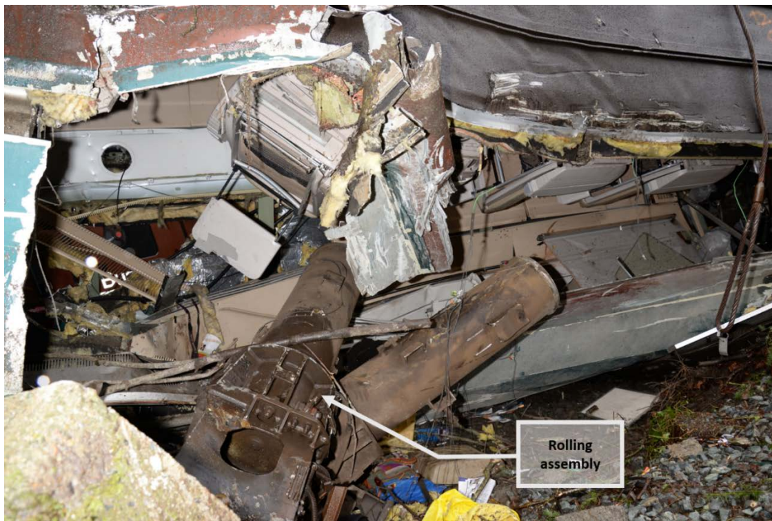
Figure 12. Detached rolling assembly tower partially inside AMTK 7504(7).
