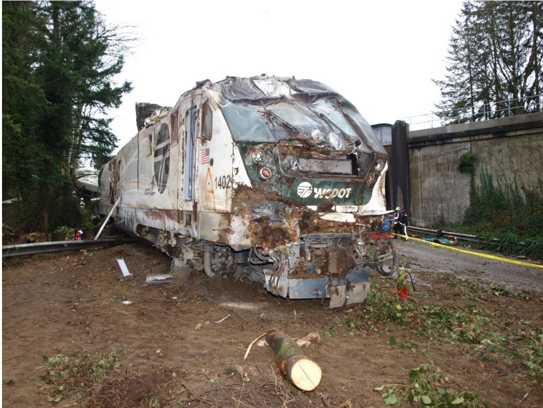
Figure 18. Damage to WDTX 1402 (1).
