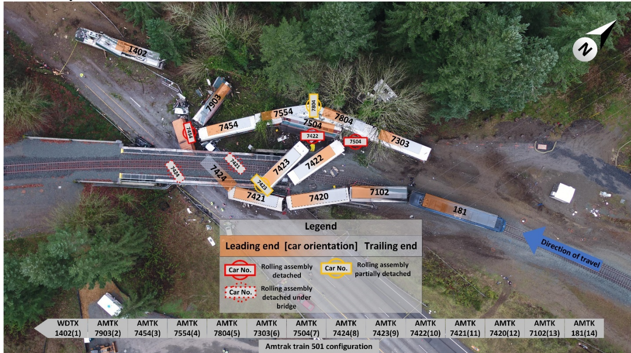
Figure 10. Overhead with railcar positions labeled. Railcar 7421 was on top of railcar 7424, which is faded because it was under the overpass. (Photo provided by WSP.)
