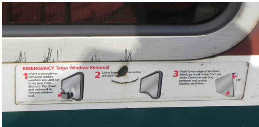
Figure 39. Interior emergency window removal instructions.
