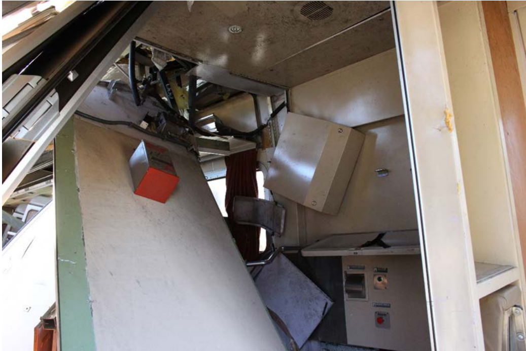
Figure 35. Photograph of the interior lavatory damage of AMTK 7504 (7).
