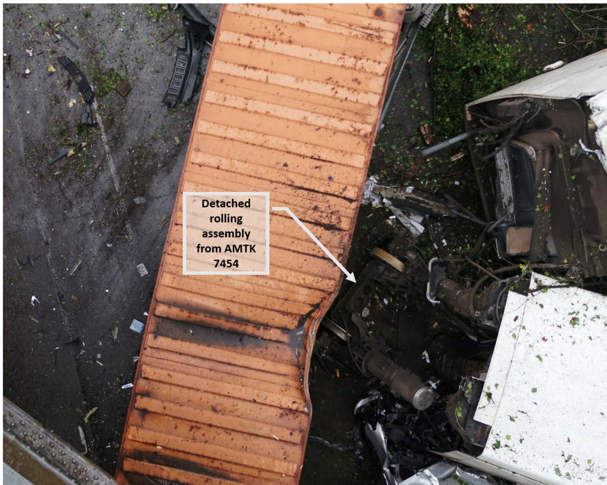
Figure 11. Detached rolling assembly from AMTK 7454 (3). (Photo provided by WSP.)
