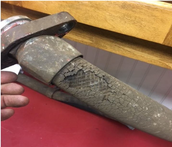
Figure 5. Close-up view of defective intermediate air brake hose removed from car LW 62114.
