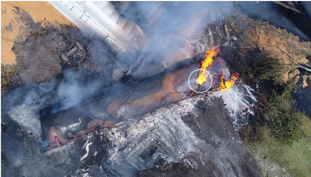
Figure 13. CBTX 781553 with puncture location circled, August 3, 2017, 2:46 p.m.
