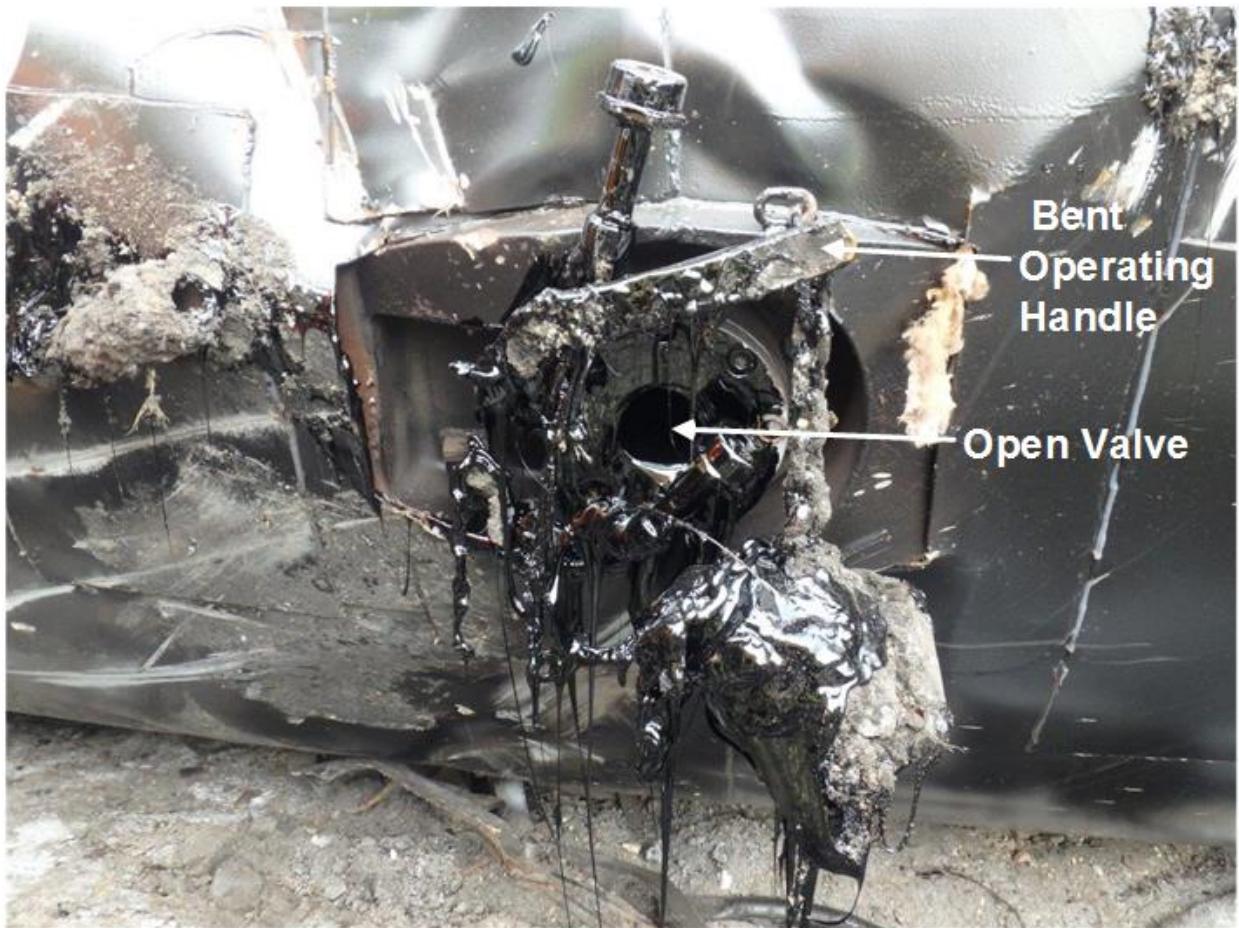
Figure 10. UTLX643949 open bottom outlet valve.
