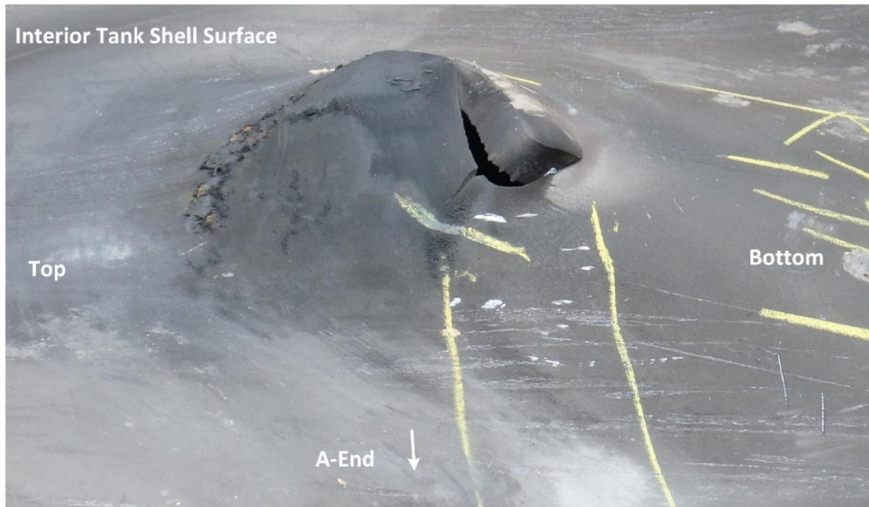
Figure 15. CTBX 781553 interior surface of shell puncture, August 5, 2017.
